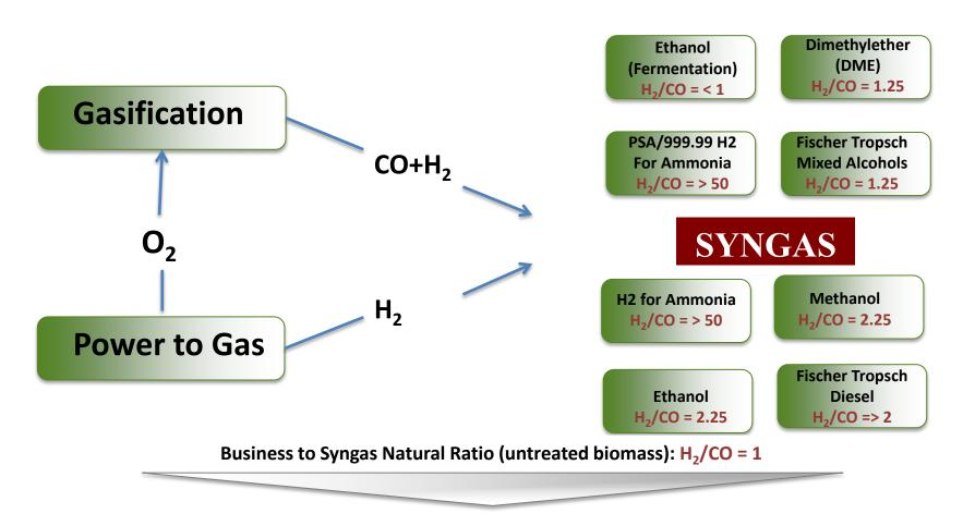
Hydrogen from P2G can optimize H2/CO ratio, residueal oxygen P2G also utilized
